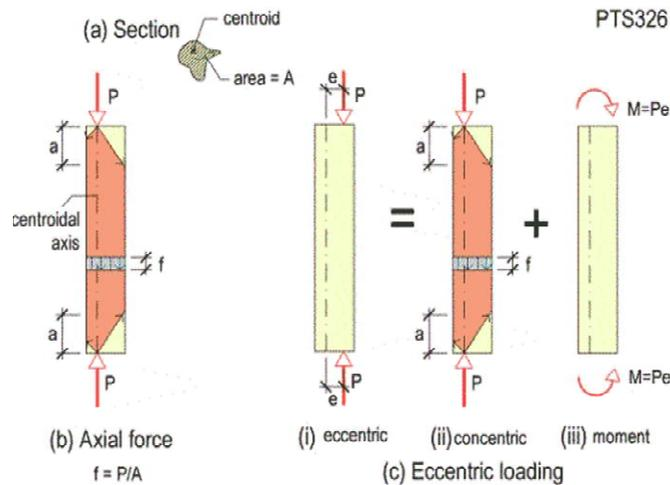
FIGURE 4.8.3.2-1 Dispersion of Force in End-Loaded Member
