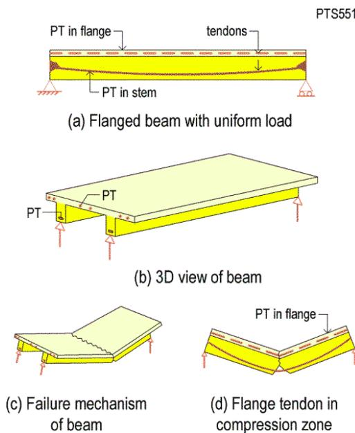
FIGURE 4.8.4-3 Flanged Beam with Tendon in Stem and Flange
