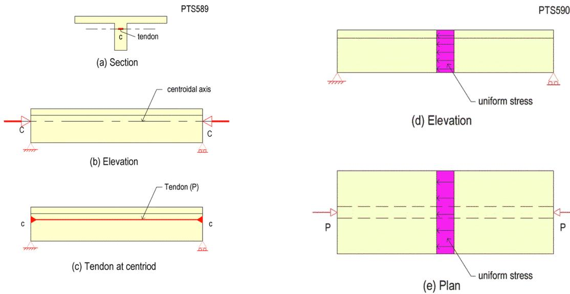
FIGURE 4.8.3.2A-2 Flanged Beam with Eccentric Tendon – Average Precompression
