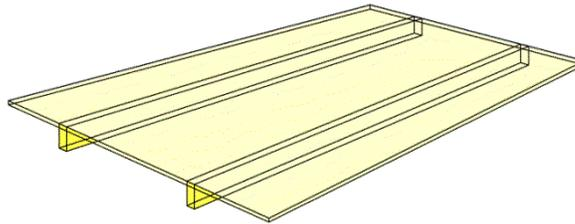
FIGURE 4.8.3.3-3 Beam and One-Way Slab Floor System
