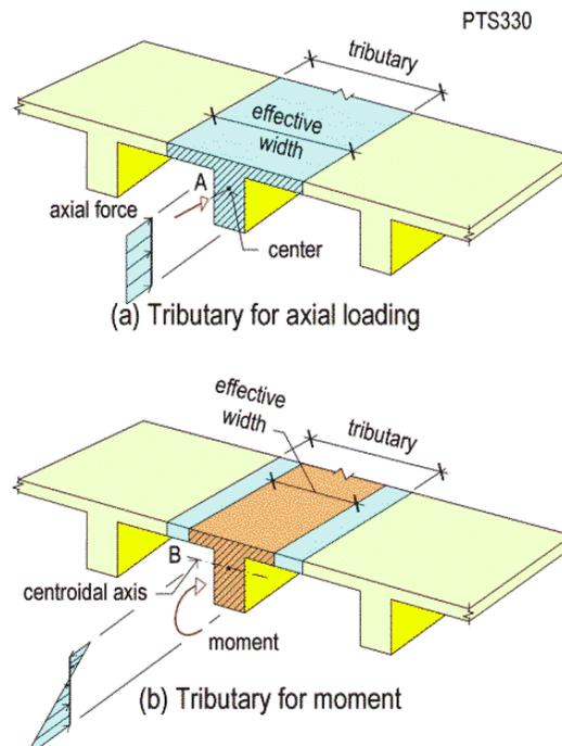
FIGURE 4.8.3.2B-1 Tributaries for Axial and Flexural Actions for Frame Analysis
