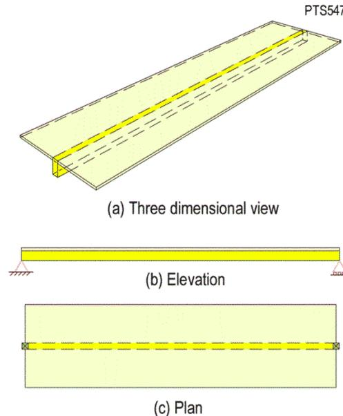
FIGURE 4.8.3.3-1 Simply Supported Flanged Beam under Uniform Loading
