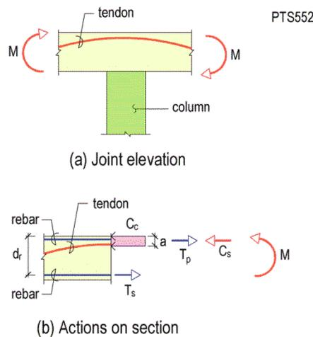
FIGURE 4.8.4-5 Force Distribution in Section with Tendon in Compression Zone
