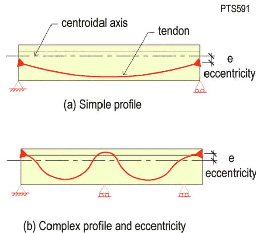
FIGURE 4.8.3.2A-3 Post-Tensioned Members with Arbitrary Tendon Profiles
