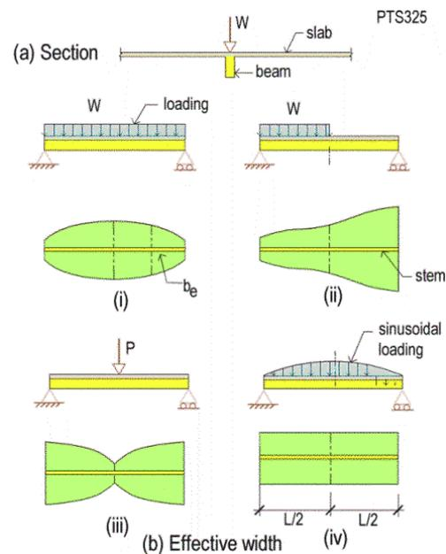
FIGURE 4.8.3.1 -2 Variation of Effective Width ( $b_e$ ) with Load
